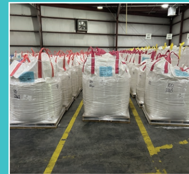
Previously, product was bagged in ‘supersacks,’ oversized plastic bags which were placed on pallets and shrink-wrapped for shipping.
