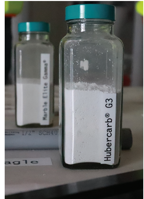
Container of Hubercarb® G3, an ultra-fine, high-purity ground calcium carbonate produced by HSM.
