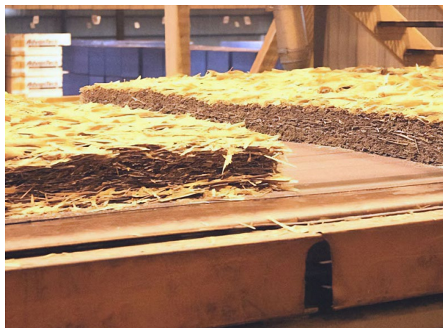
A master mat of the oriented strand about to enter the press to become the premium brand of OSB, AdvanTech® subflooring.
